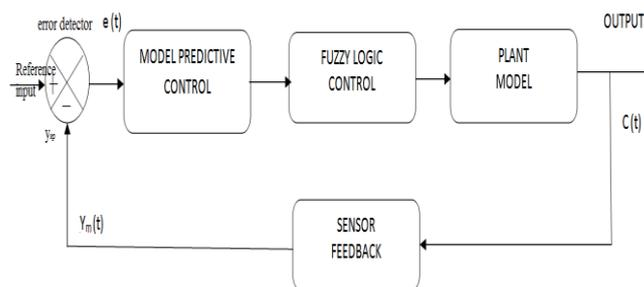
Fig.3 proposed controller design for temperature process
