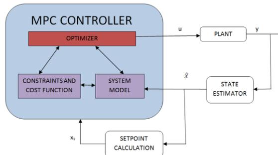
Fig.1 Basic Structure of MPC
